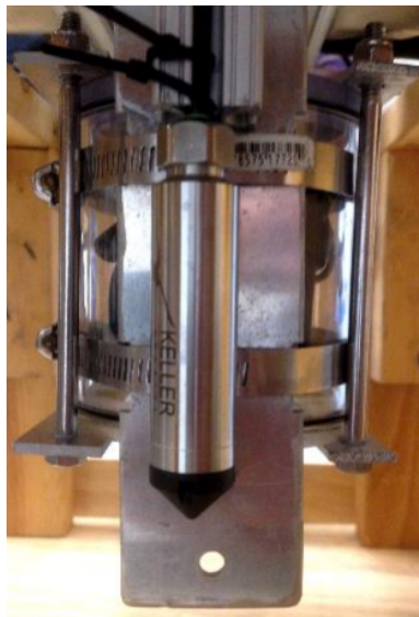
Figure 8: Depth Sensor and Mounting on Bottom Camera
